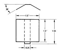
Staver Heat Sink #V-7 Staver Company 41 Saxon Ave. P.O. Drawer H Bayshore, NY 11706 Tel: (516) 666-8000 Copper Wings 2 Required Soldered to Pins 3, 4, 5, 10, 11, 12 Thickness 0.04 Inches
